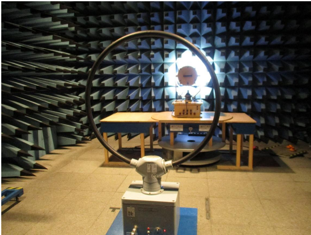
Figure 5: Test set-up EUT 01, 150 kHz to 30 MHz
